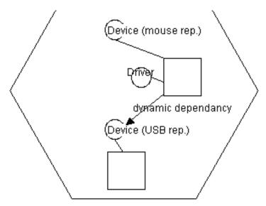
Thus the physical mouse device is represented by two Device services. The bottom one represents the mouse in a generic USB form, while the upper represents it specifically as a mouse. The USB driver discovers new physical devices by interacting with software support outside of the OSGi environment. The upper driver has registered a
